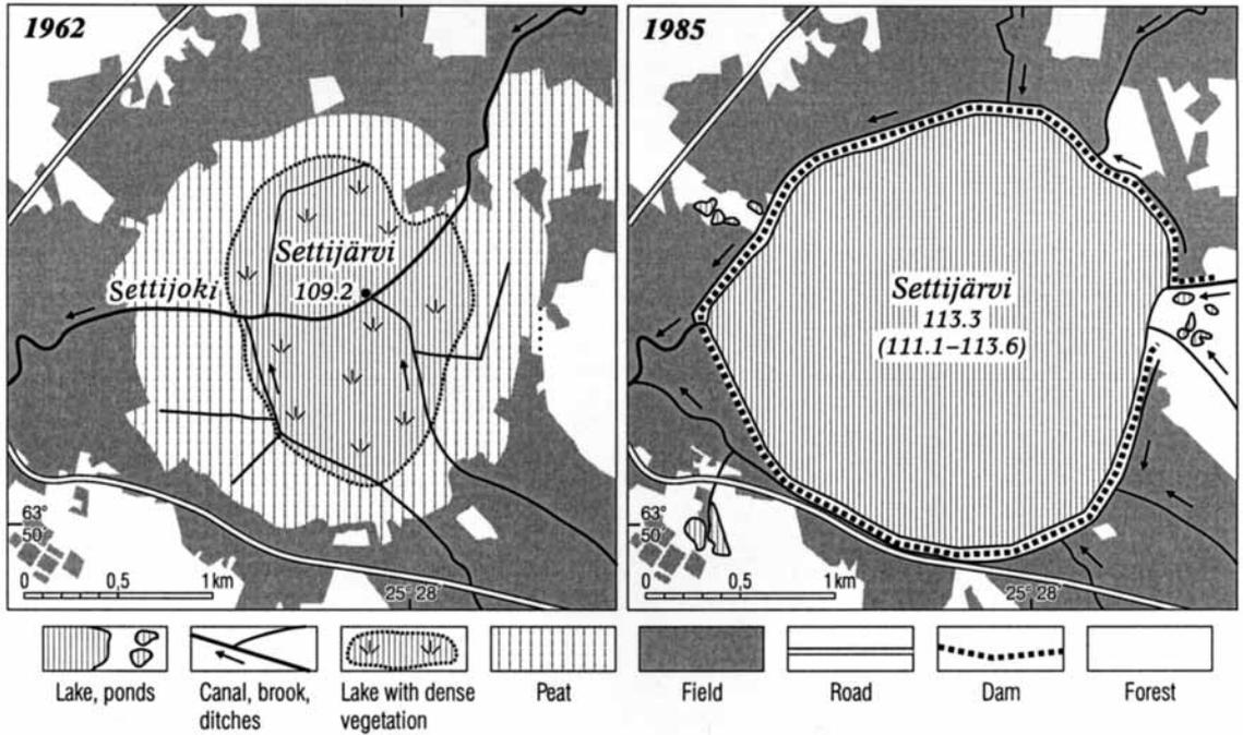
Fig. 4. Lake Settijärvi in Haapajärvi before and after damming and regulation.
